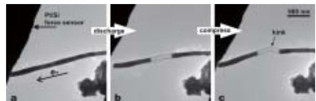
Fig. 3. (a) C tube filled with Zn(Ga)S. The current (e-) causes Joule heating which leads to the core discharge; (b) tube seen in (a) after partial removal of its core. (c) Plastic deformation of the emptied, and thus weakened structure fragment, under compression in TEM.
