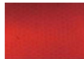
**Fig.3.** Fluorescent image. Film thickness of ~150 nm, excitation at 535- 565 nm, emission at 590 nm.
