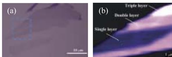
Figure 1. (a) Optical microscope image of graphene flakes on  $\text{SiO}_2/\text{Si}$ . (b) Raman mapping of the integrated intensity of G-band Raman peak in the dashed square region in (a).
